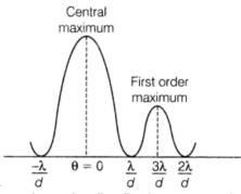
Intensity distribution curve and diffraction pattern due to single slit
